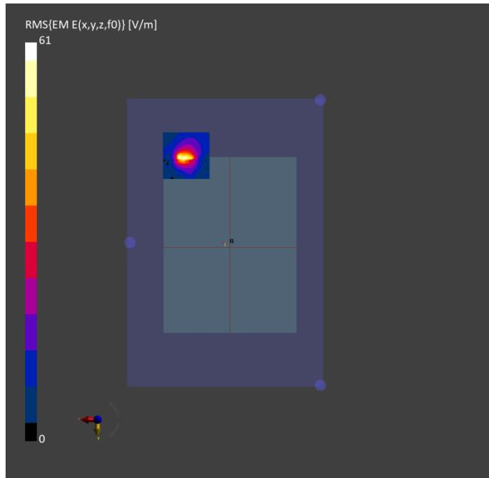
**6. SAR System Check From 6500MHz****Exposure Conditions**
