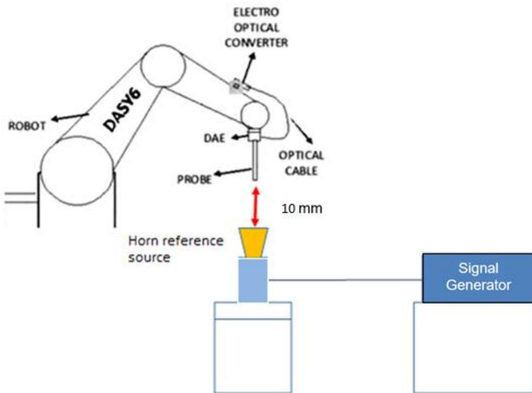
The output power on the reference source is set to 22.0 dBm (158.49 mW) and the measurement results Avg PD for 4cm<sup>2</sup> are compared with the power density targets on the calibration certificate.
