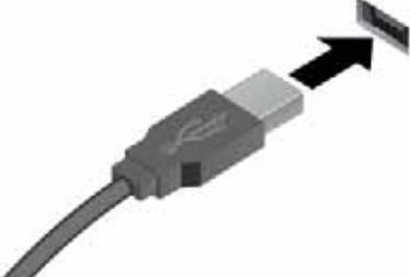
A standard rectangular USB-A connector with a black arrow pointing to its top edge.                                                  | Connect USB-compatible devices, such as a USB keyboard, USB mouse, USB storage device, or USB printer.
