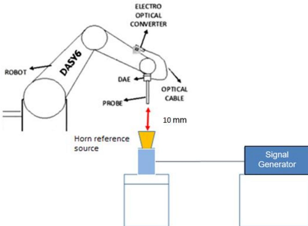
The output power on the reference source is set to 22.0 dBm (158.49 mW) and the measurement results Avg PD for  $4\text{cm}^2$  are compared with the power density targets on the calibration certificate.
