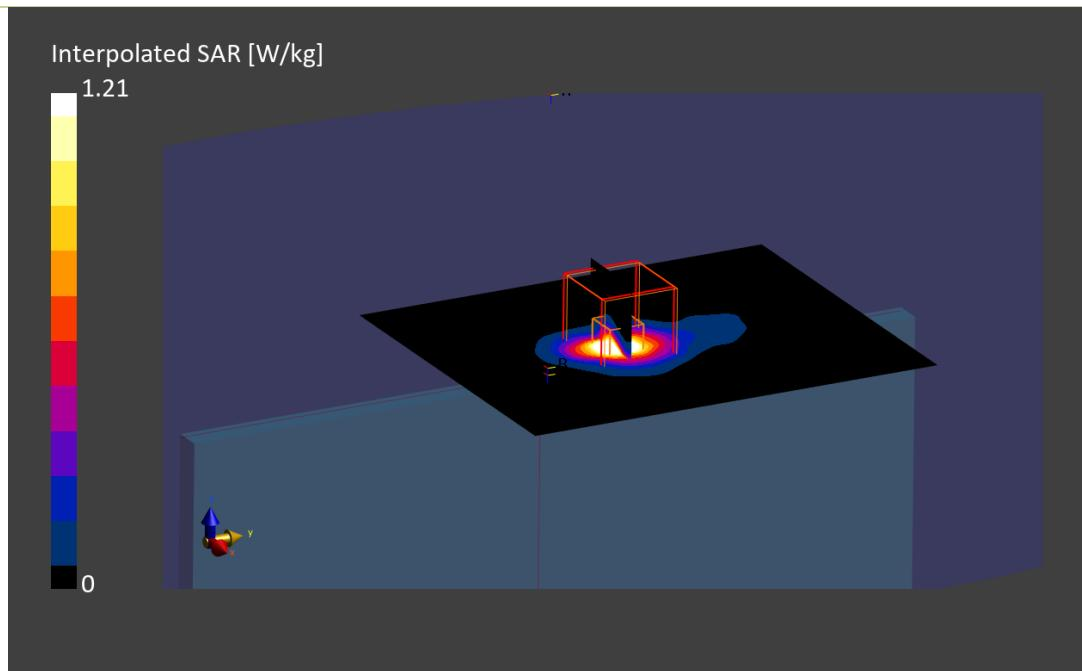
**5. U-NII-4 - 802.11ac160, CH163, Aux Antenna –Bottom edge– Vendor 2****Device under Test Properties**
