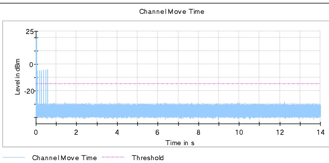
**Channel move time < 10s, test PASS**
