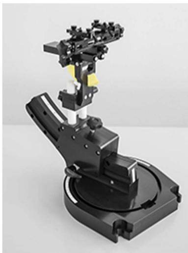
The DASY device holder is designed to cope with the different positions given in the standard. It has two scales for device rotation (with respect to the body axis) and device inclination (with respect to the line between the ear reference points). The rotation center for both scales is the ear reference point (ERP). Thus the device needs no repositioning when changing the angles.
