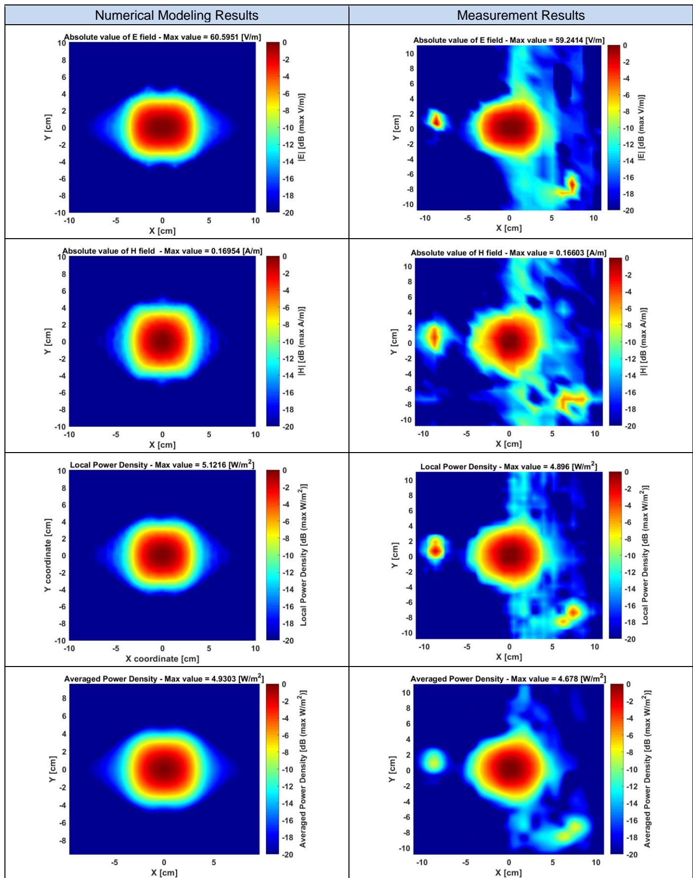
The plots below show the comparison between the numerical modeling and the system check results in terms of normalized E-field distribution and the 1D variation along the two axis of the maximum.
