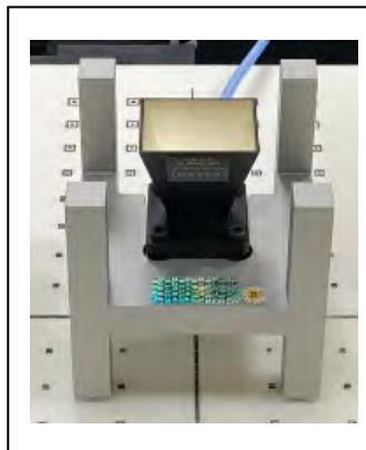
The verification sources apply to system check or verification at specific mmWave frequencies. The sources comprise horn-antennas and very stable signal generators.
