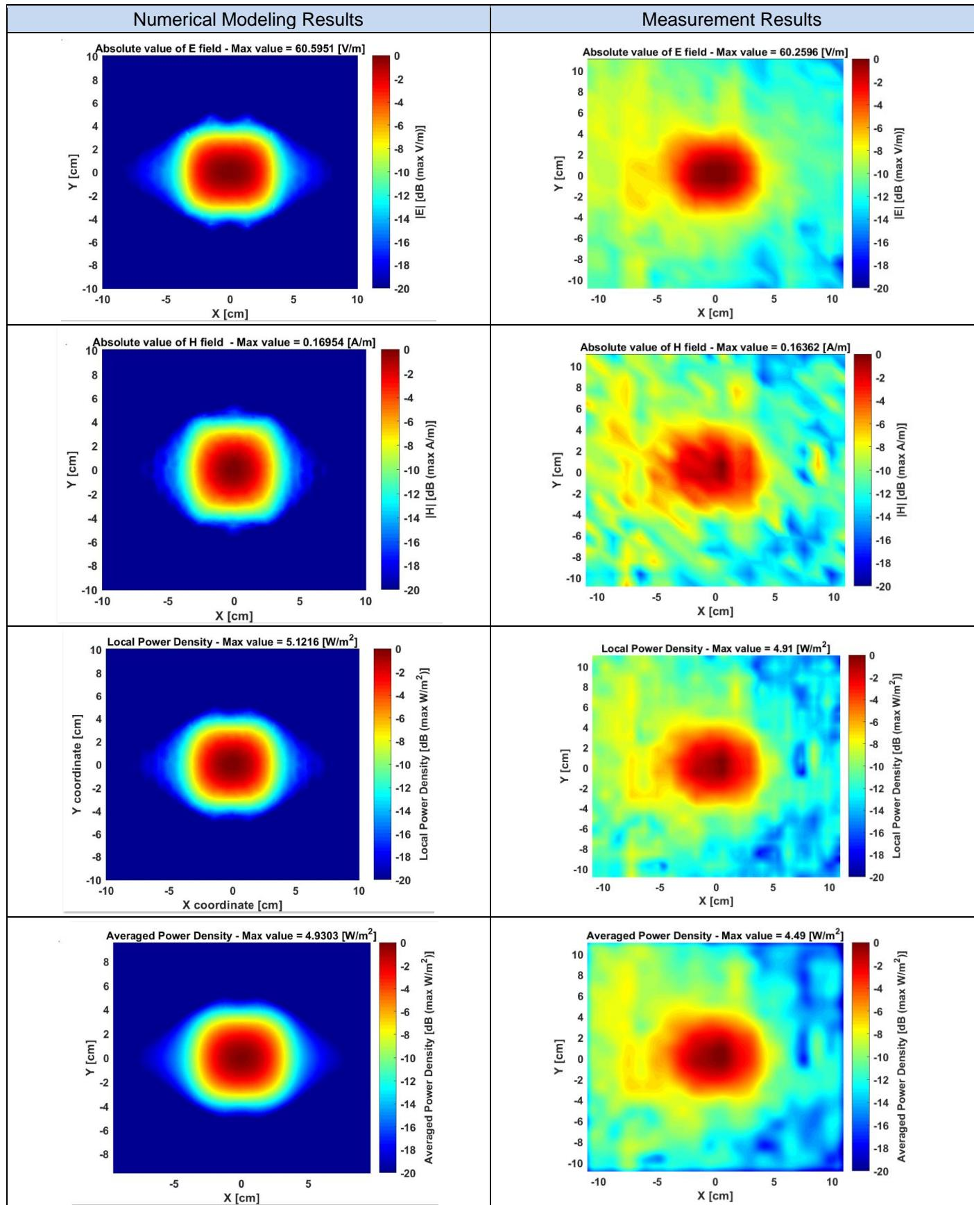
The plots below show the comparison between the numerical modeling and the system check results in terms of normalized E-field distribution and the 1D variation along the two axis of the maximum.
