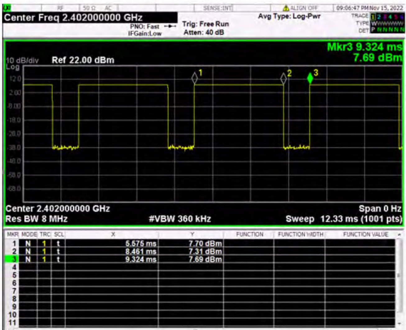
Time-domain plot for Bluetooth transmission signal
