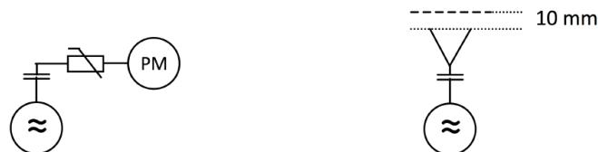
First, the power meter is connected to the output of the signal generator to measure the forward power at the location of the connector to the system check source. The signal generator is adjusted for the desired forward power to match the system check source calibration setup at the connector as read by power meter. Then the power meter is replaced by the system check source.
