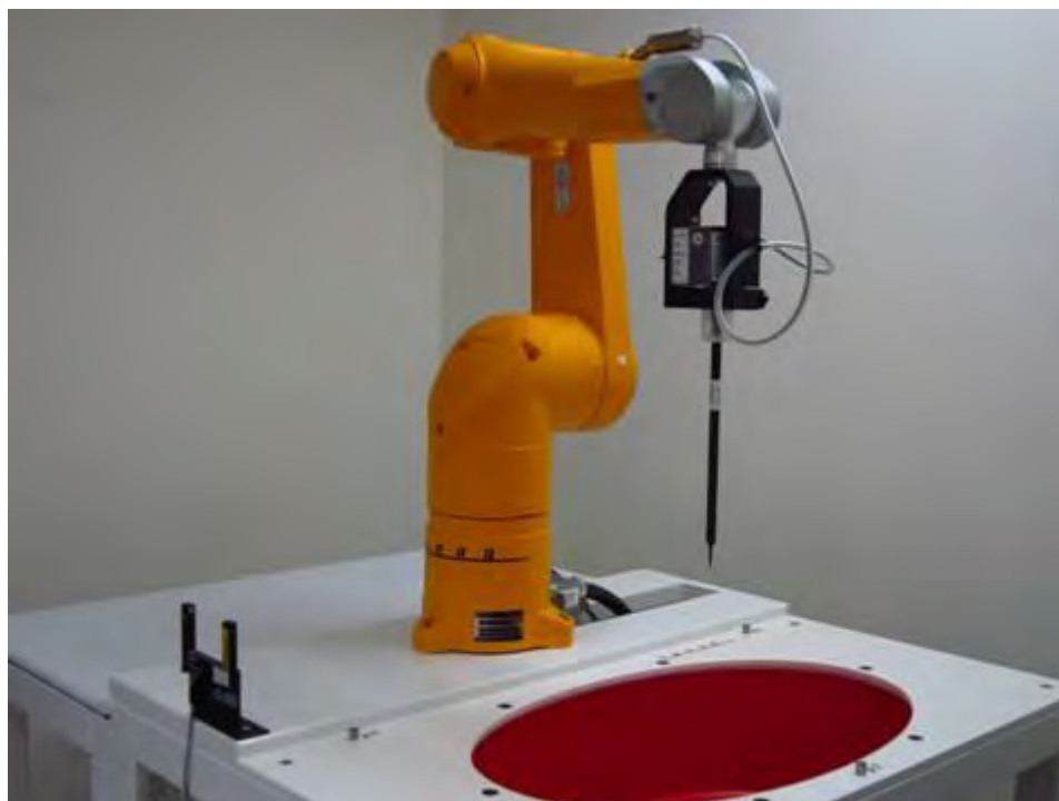
Fig.1 Photograph of the SAR measurement system
