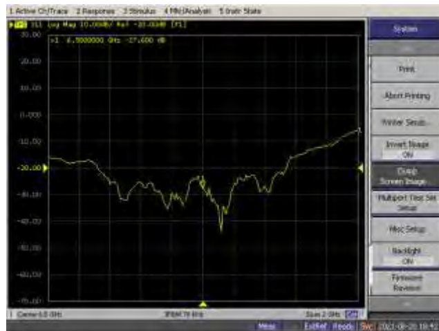
< Figure 1. Measurement result of Head Return Loss >
