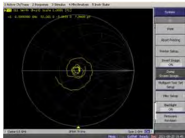
< Figure 2. Measurement result of Head Impedance >
