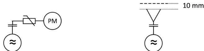
First, the power meter is connected to the output of the signal generator to measure the forward power at the location of the connector to the system check source. The signal generator is adjusted for the desired forward power to match the system check source calibration setup at the connector as read by power meter. Then the power meter is replaced by the system check source.
