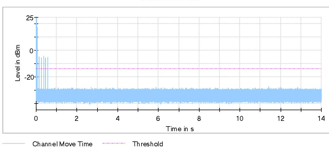
**Channel move time < 10s, test PASS**
