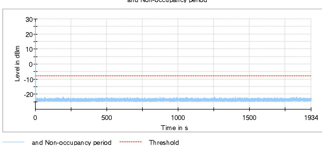
**No transmission of any type has occurred for 30 minutes, test PASS**
