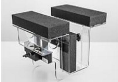
The DASY device holder is designed to cope with the different positions given in the standard. It has two scales for device rotation (with respect to the body axis) and device inclination (with respect to the line between the ear reference points). The rotation center for both scales is the ear reference point (ERP). Thus the device needs no repositioning when changing the angles.
