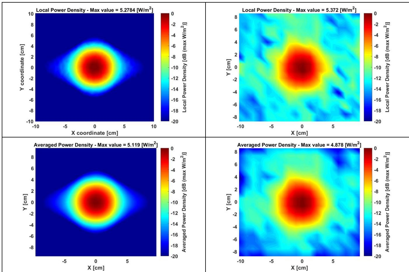
The plots below show the comparison between the numerical modeling and the system check results in terms of normalized E-field distribution and the 1D variation along the two axis of the maximum.
