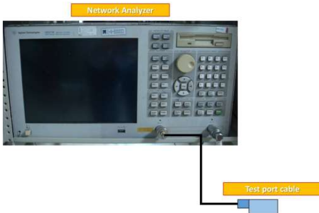
Figure 1. The schematic diagram for measuring VSWR
