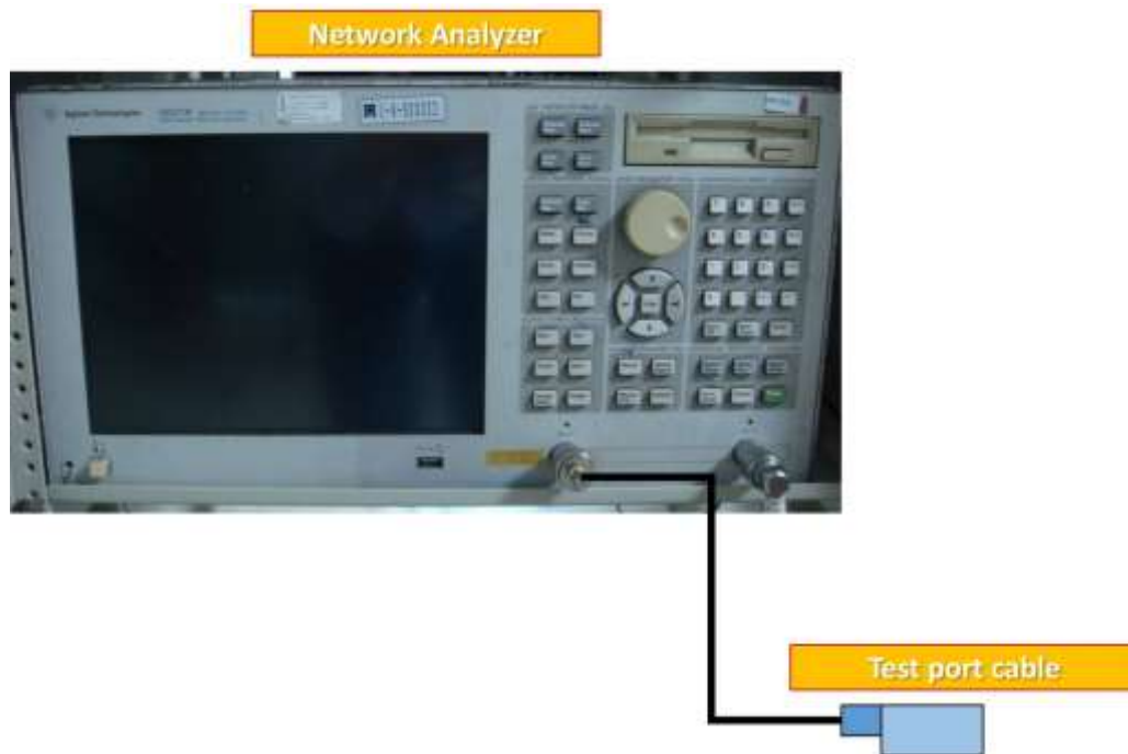
Figure 1. The schematic diagram for measuring VSWR
