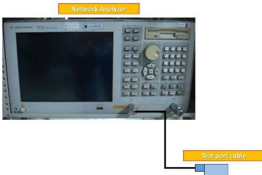
Figure 1. The schematic diagram for measuring VSWR
