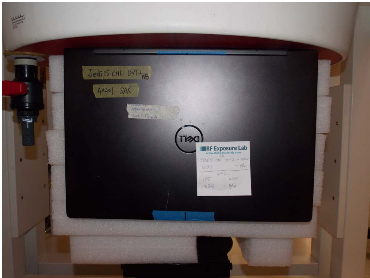
Test Position Laptop 0 mm Gap
