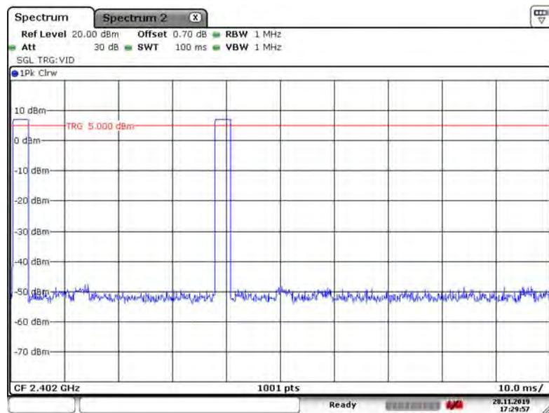
Time on of 100ms=  $2.87\text{ms} \times 2 = 5.74\text{ms}$
