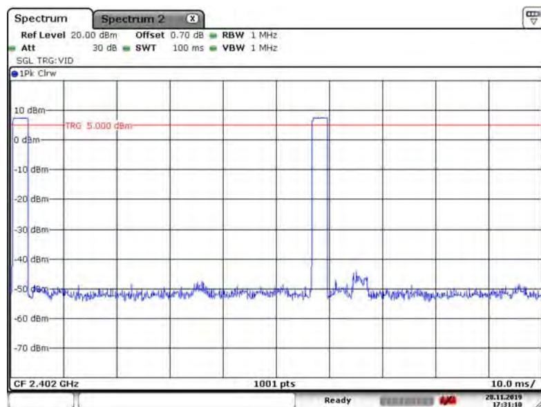
Time on of 100ms=  $2.88\text{ms} \times 2 = 5.76\text{ms}$
