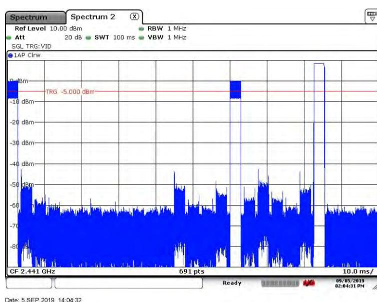
Time on of 100ms=  $2.884\text{ms} \times 3 = 8.652\text{ms}$
