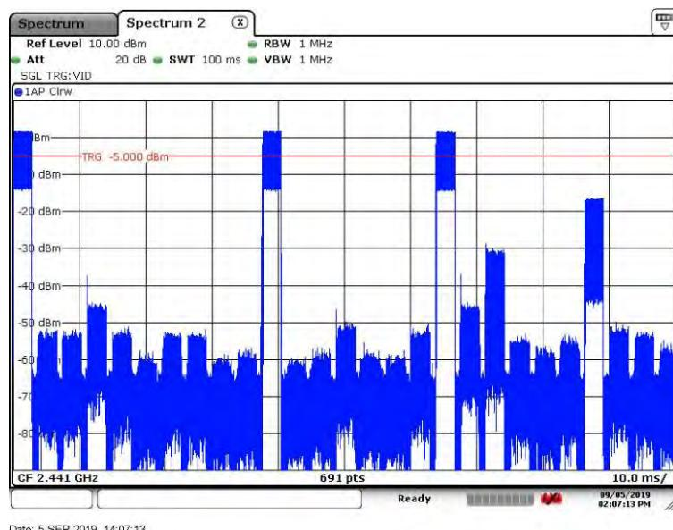
Time on of 100ms=  $2.898\text{ms} \times 3 = 8.694\text{ms}$
