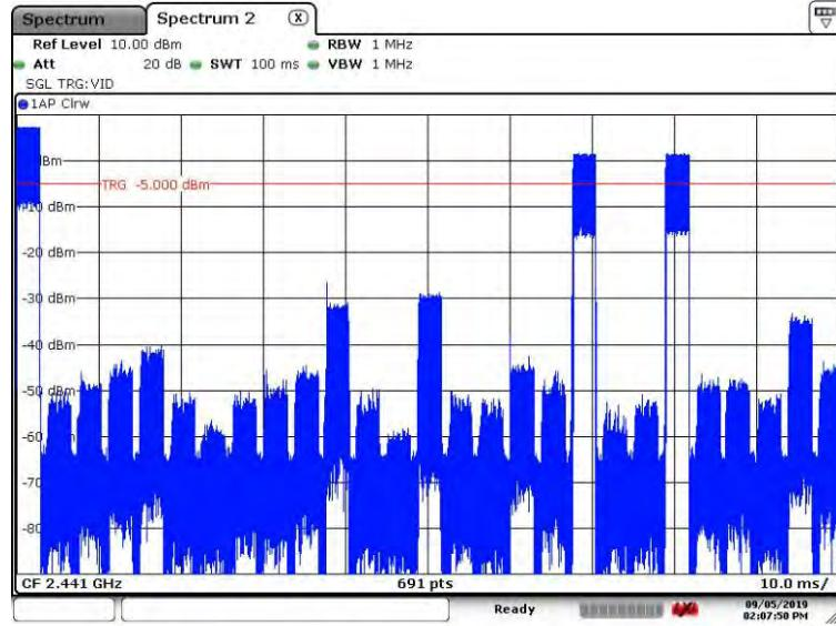
Time on of 100ms=  $2.89\text{ms} \times 3 = 8.694\text{ms}$ Duty Cycle=  $8.694\text{ms} / 100\text{ms} = 0.08694$ Duty Cycle correction factor=  $20 \text{ LOG } 0.08694 = -21.216 \text{ dB}$
