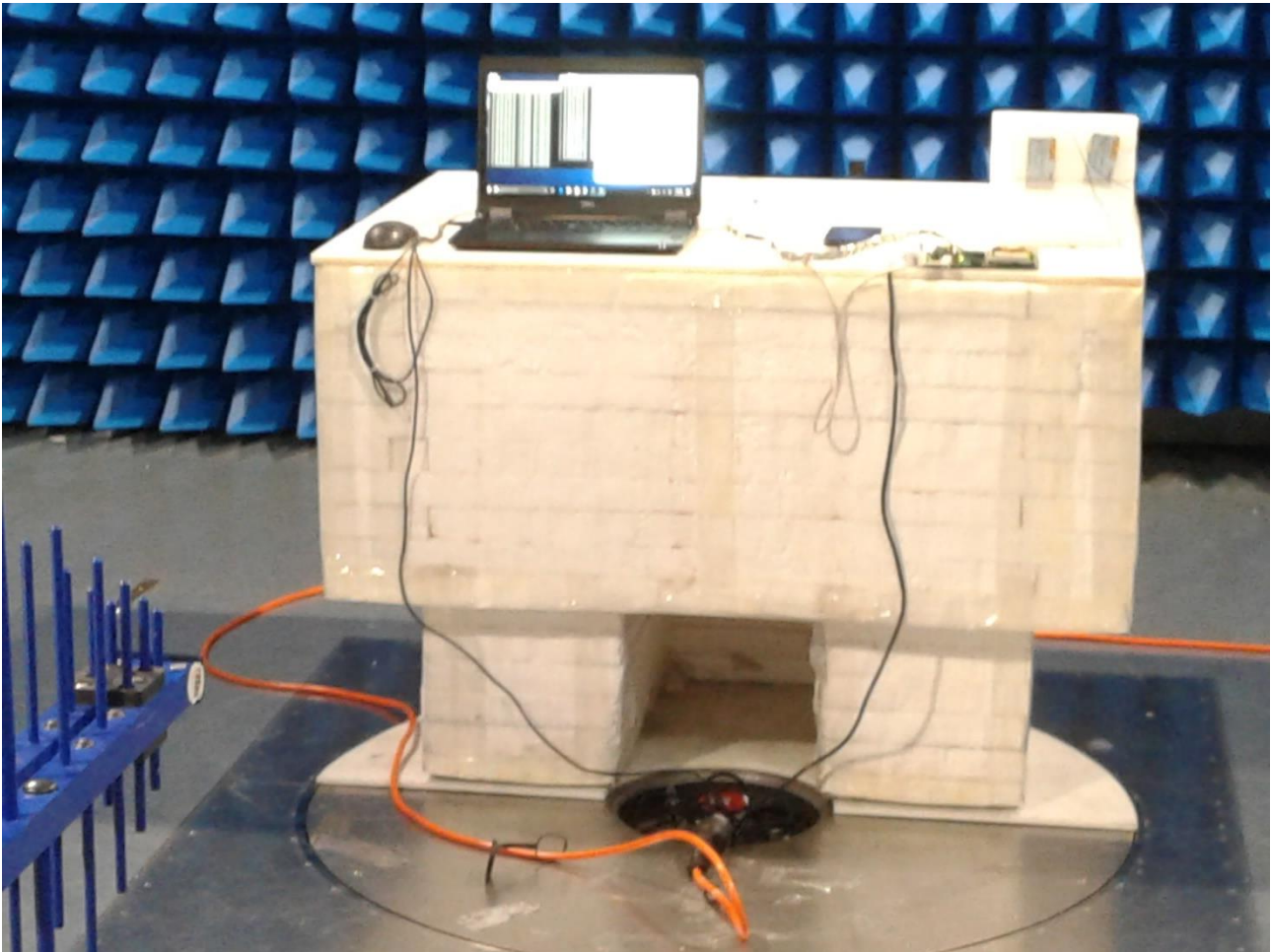
Photo 1 Photograph test setup radiated emissions 30-1000 MHz
