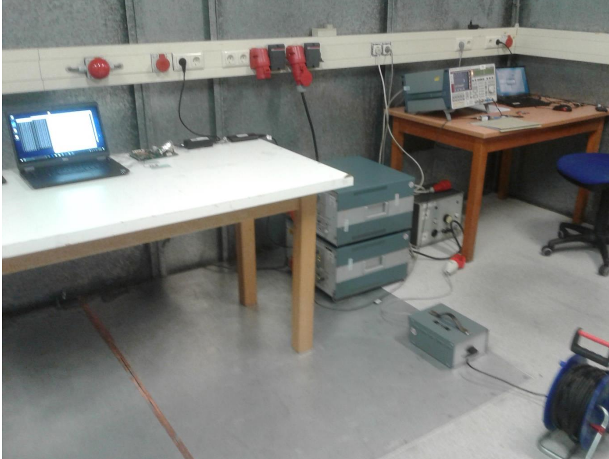
Photo 5: Photograph conducted emissions 0.15-30 MHz
