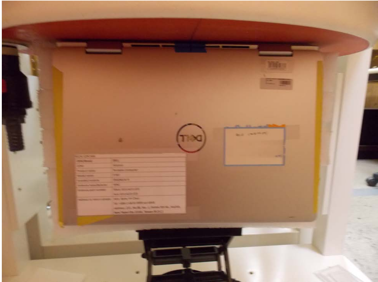
Test Position Laptop 0 mm Gap
