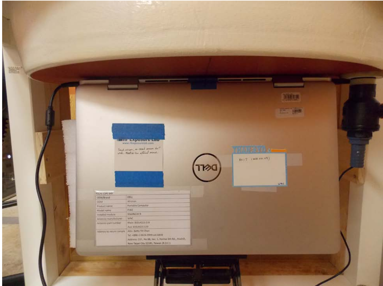
Test Position Laptop 0 mm Gap
