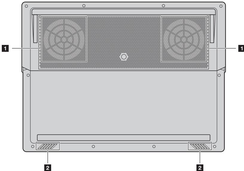
**1 Louvers** Allow air to enter the computer for cooling.
