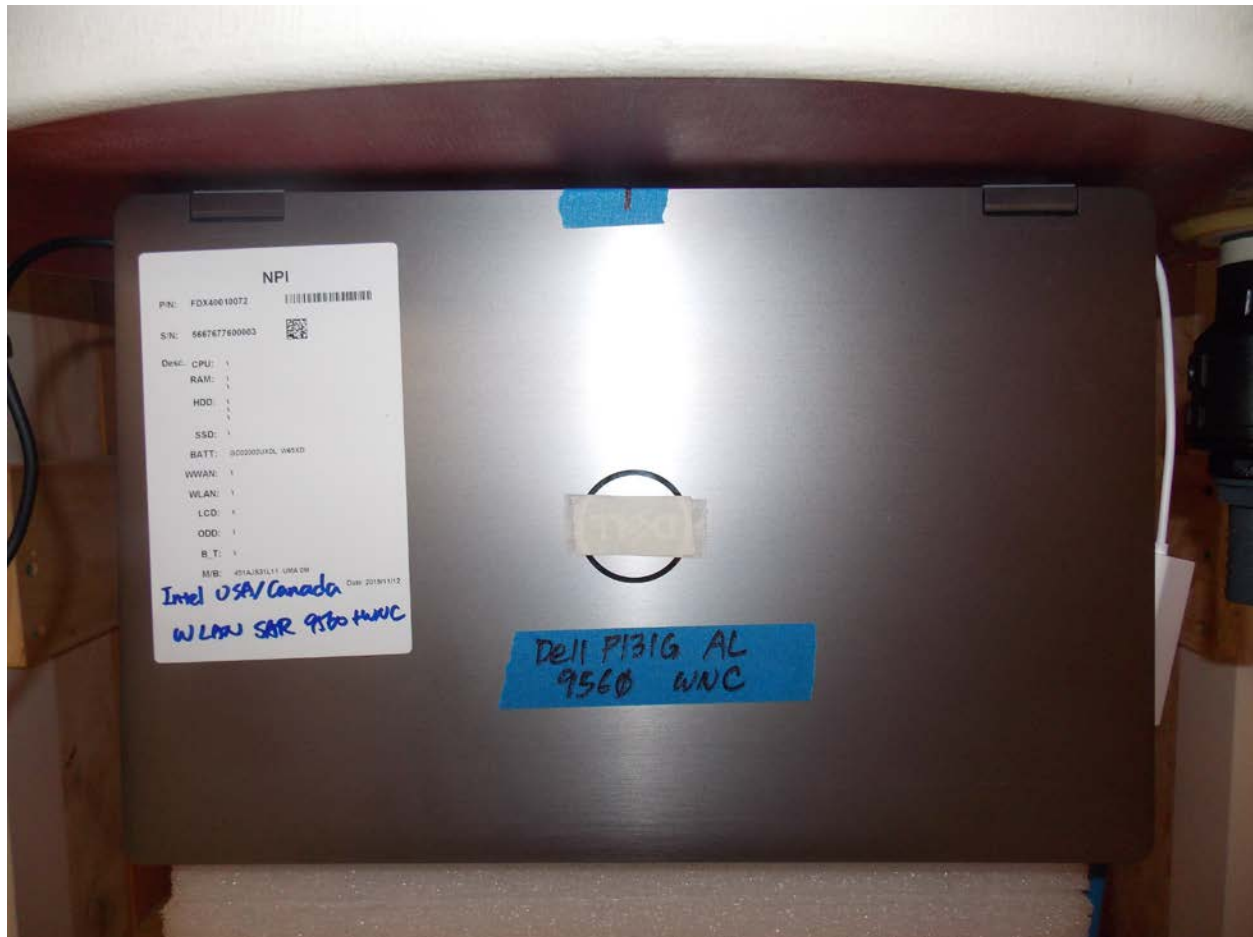
Test Position Laptop 0 mm Gap
