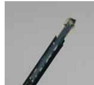
EX3DV4 E-Field Probe
