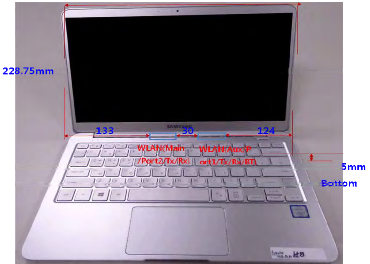
<The Distance information of Antenna to Edges of Notebook>
