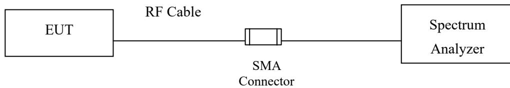
**Conduction Power Measurement (for 802.11an)**
