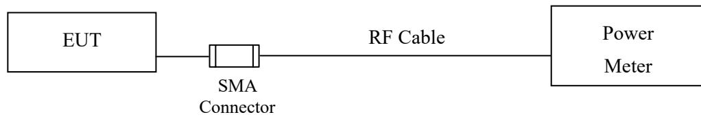
**Conduction Power Measurement (for 802.11ac)**
