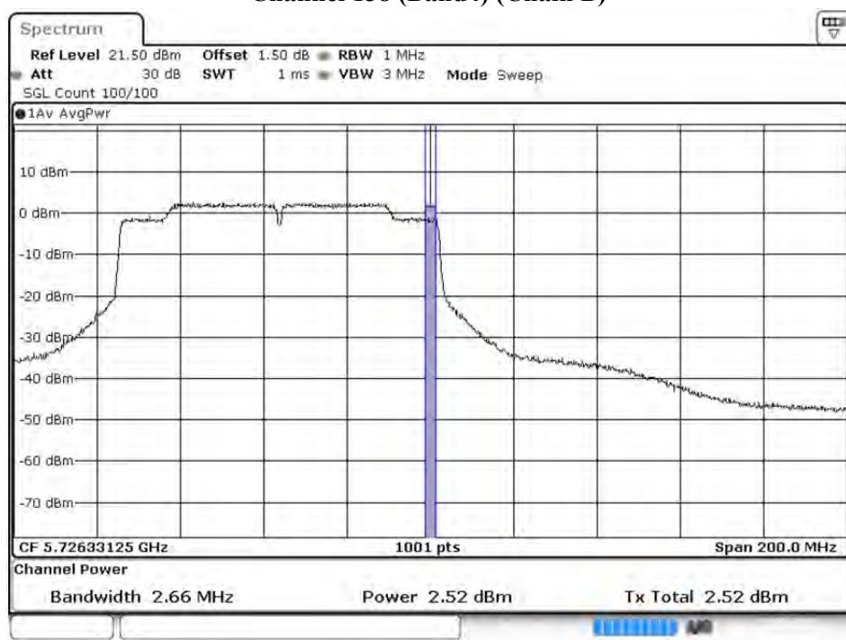
**Maximum conducted output power:****Channel 155 (Chain A)**
