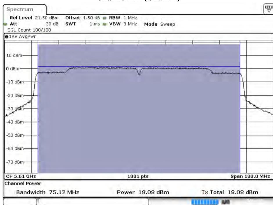
**Maximum conducted output power:****Channel 138 (Band3) (Chain A)**
