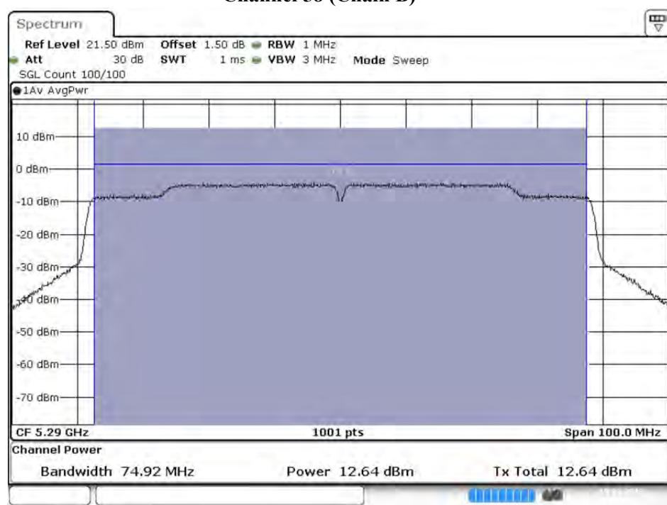
**Maximum conducted output power:****Channel 106 (Chain A)**
