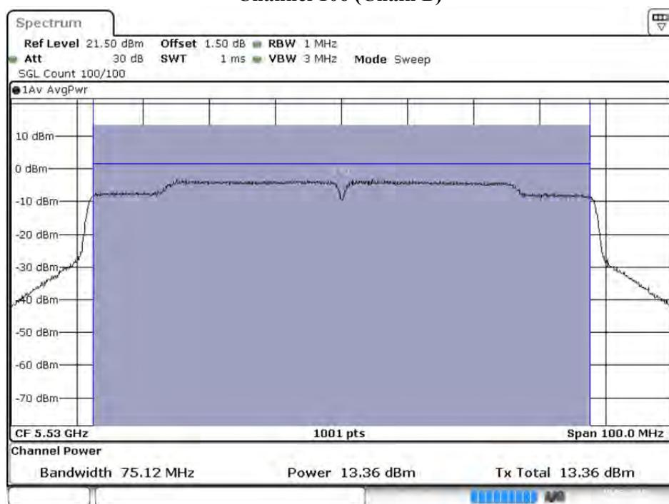
**Maximum conducted output power:****Channel 122 (Chain A)**
