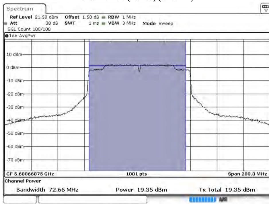
**Maximum conducted output power:****Channel 138 (Band4) (Chain A)**
