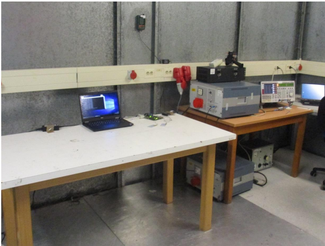
Photo 5: Test Set-up Conducted emission 0.15 MHz to 30Mhz
