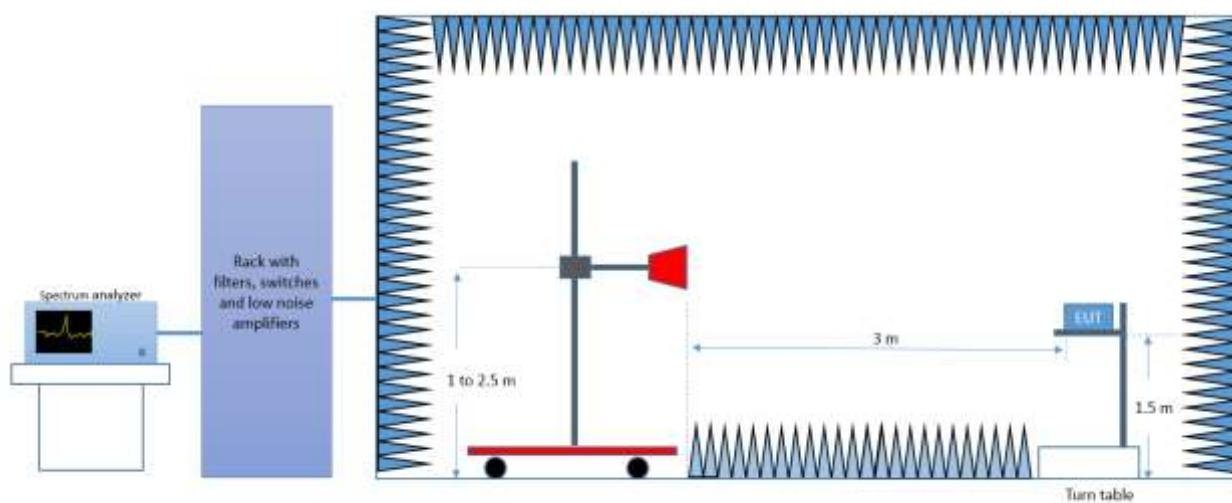
*Radiated Setup 6.4 GHz - 18 GHz*
