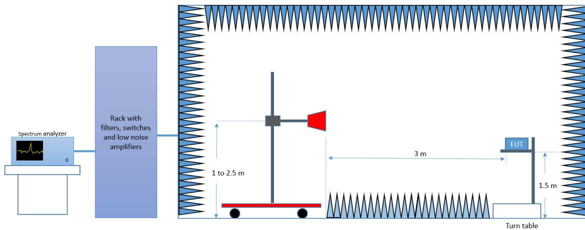
*Radiated Setup 18 GHz - 40 GHz*
