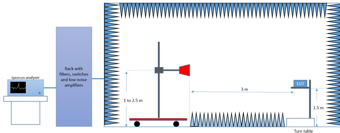
*Radiated Setup 18 GHz – 40 GHz*
