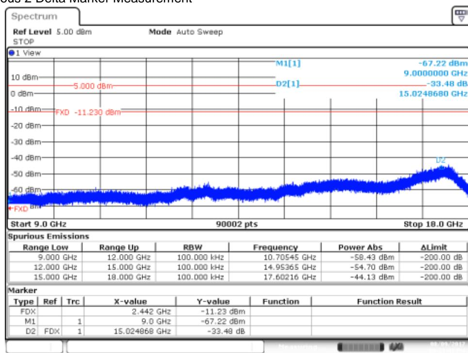
Channel 7 - Spurious 3 Delta Marker Measurement
