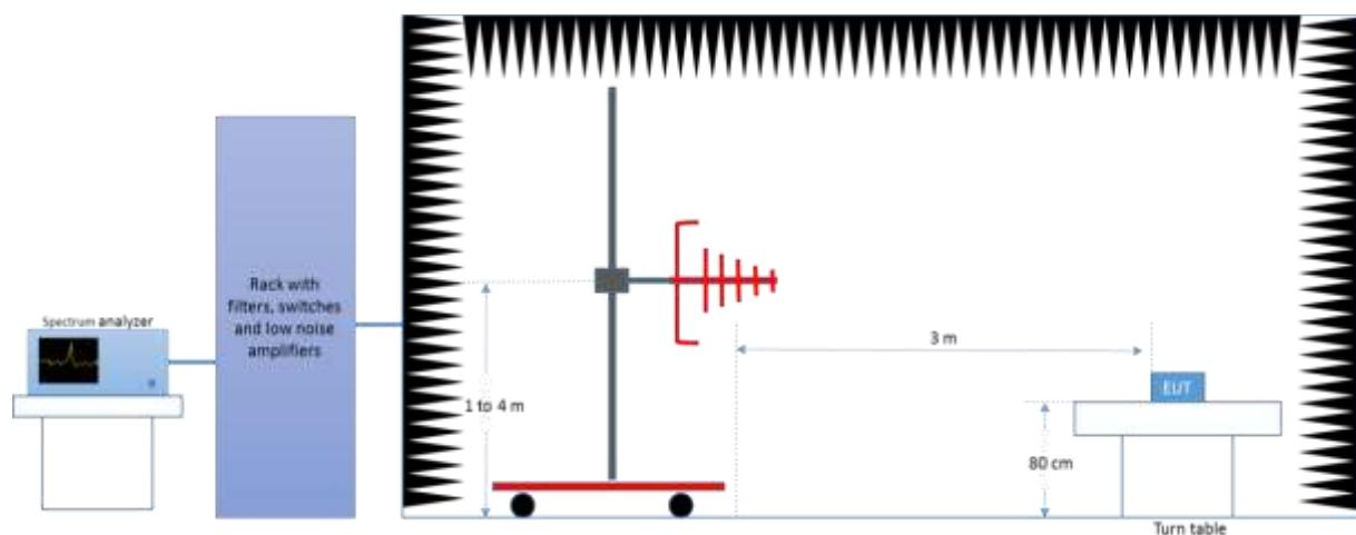
*Radiated Setup 1 GHz - 18 GHz*
