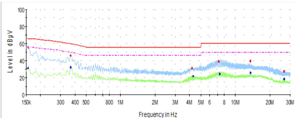
— Peak measurements — Avg measurements — Limit FCC Quasi-Peak - - - Limit FCC Avg
