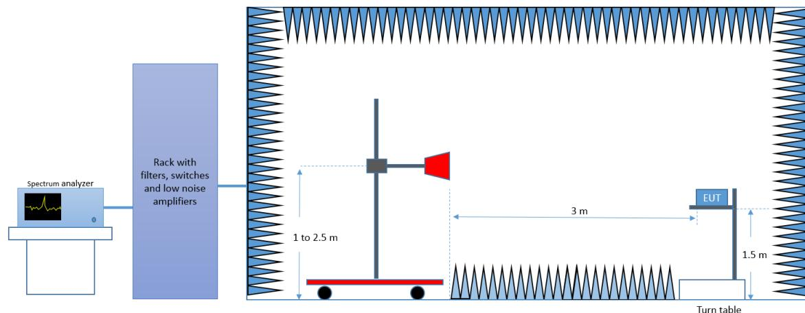
*Radiated Setup 18 GHz – 25 GHz*
