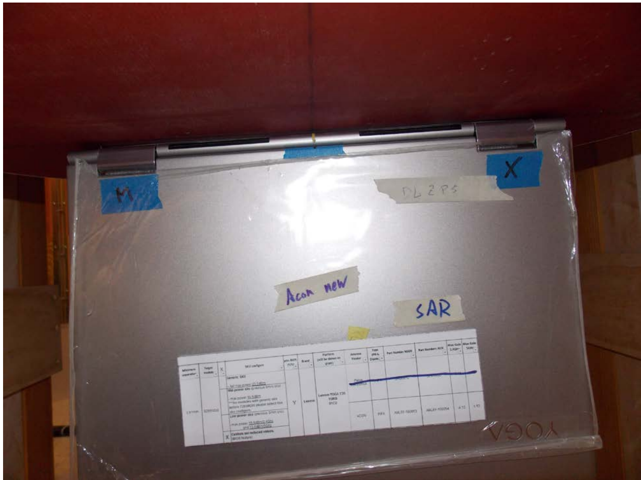
Test Position Laptop 0 mm Gap
