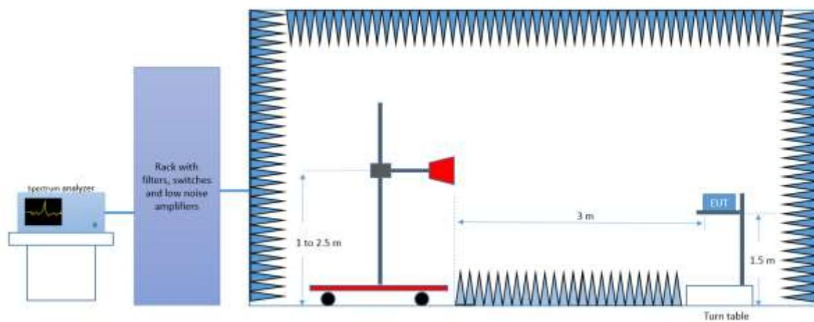
*Radiated Setup 18 GHz - 40 GHz*
