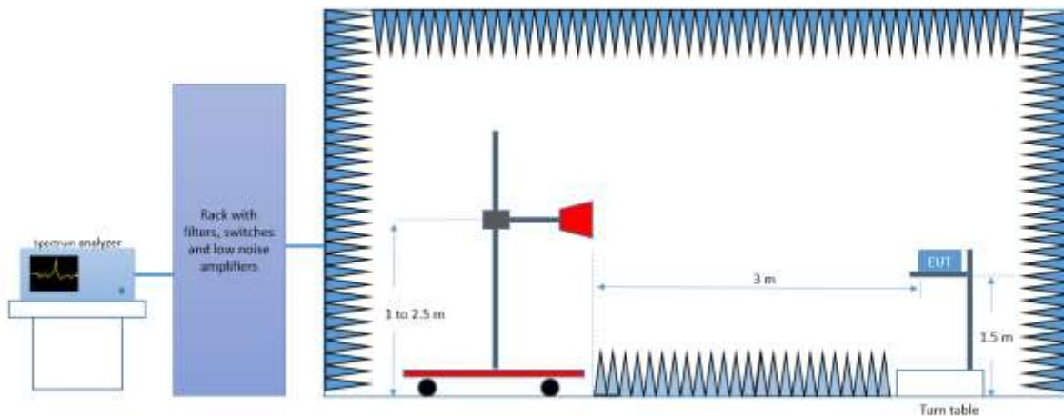
*Radiated Setup 18 GHz – 40 GHz*
