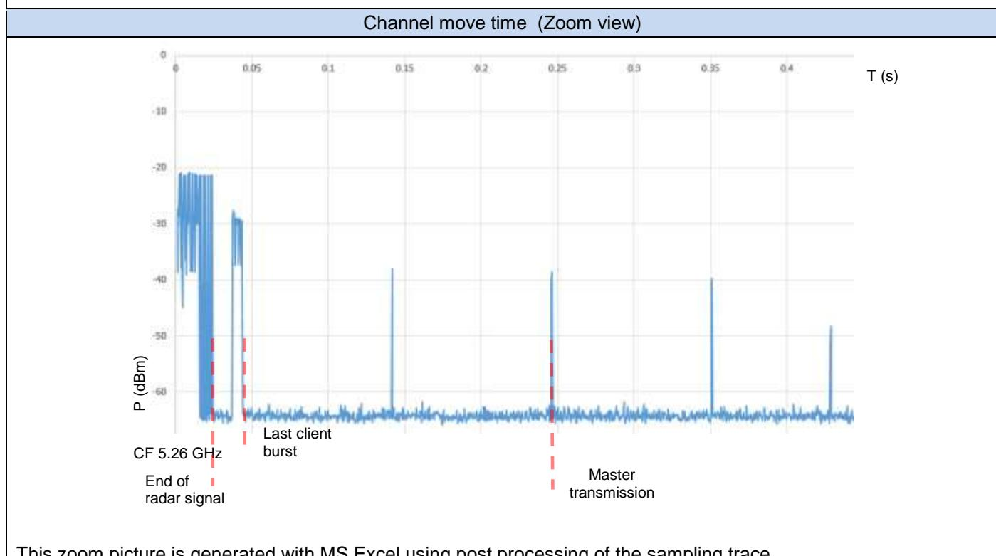
This zoom picture is generated with MS Excel using post processing of the sampling trace.
