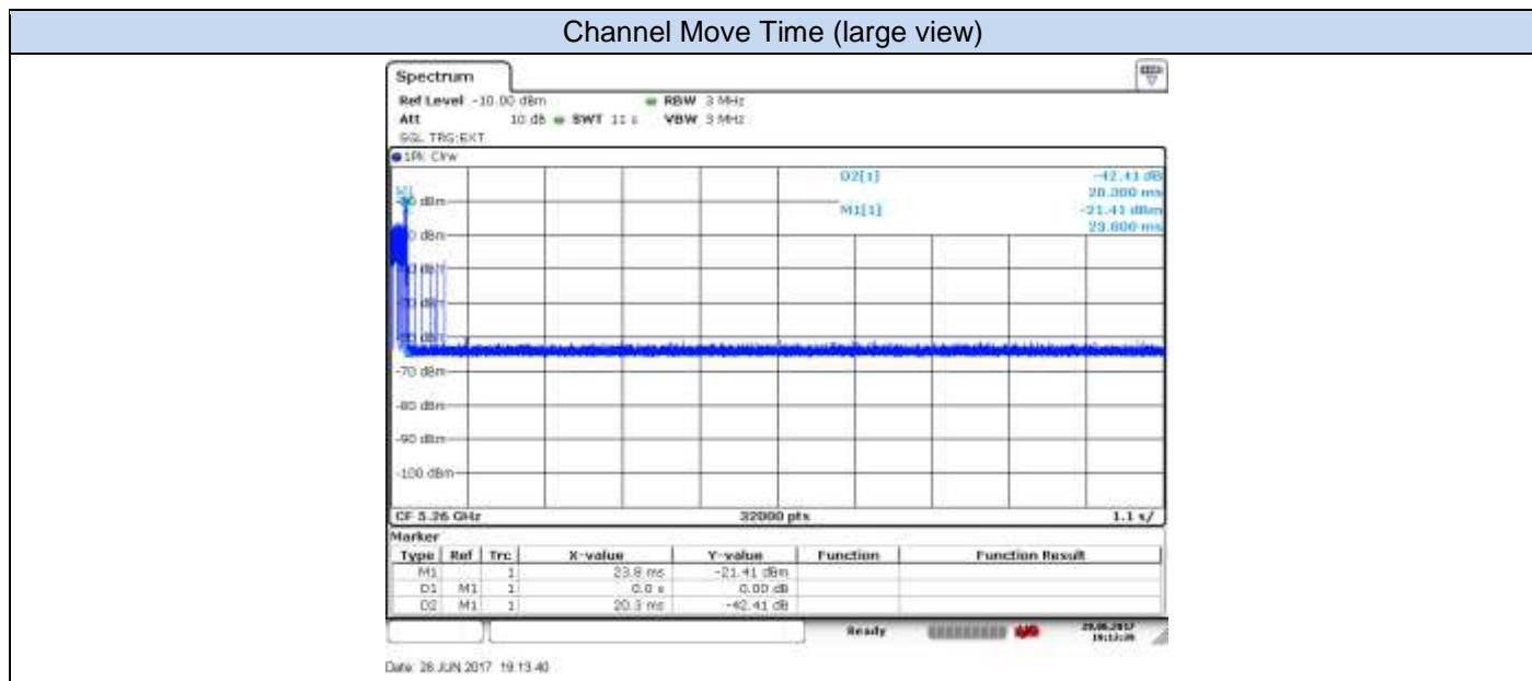
**Marker M1 shows the end of the radar signal.**
