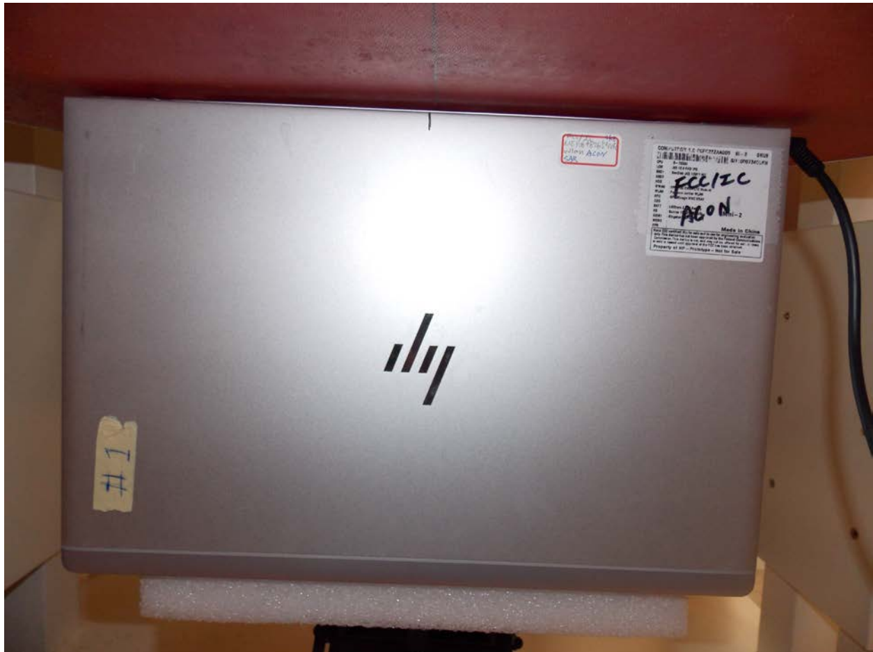
Test Position Laptop Mode 0 mm Gap
