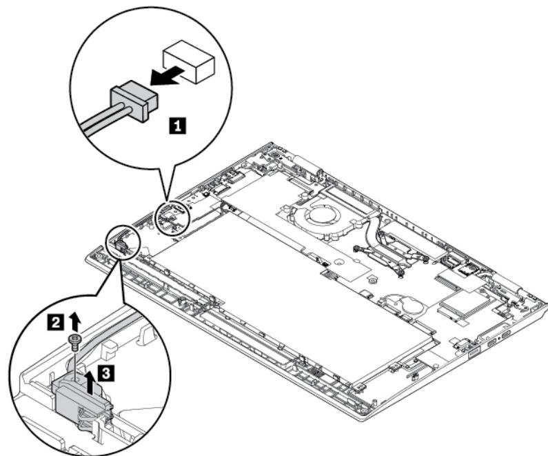
6. Install the screw to secure the pen charger. Then, connect the connector to the system board.
