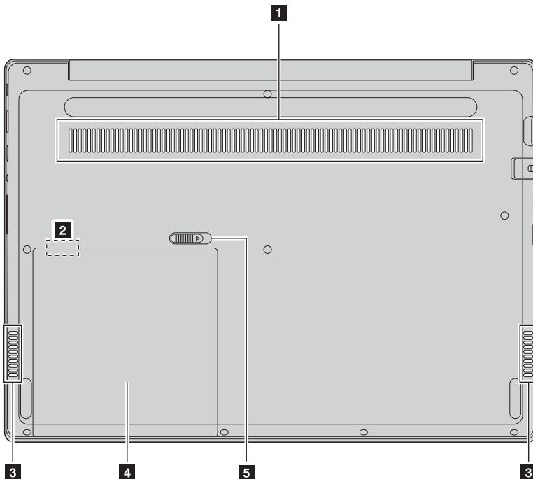
**1 Ventilation slots** Dissipate internal heat.
