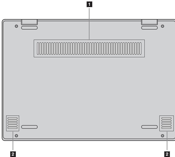
**1 Louvers** Allow air to enter the computer for cooling.
