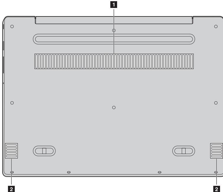
**[1] Louvers** Allow air to enter the computer for cooling.
