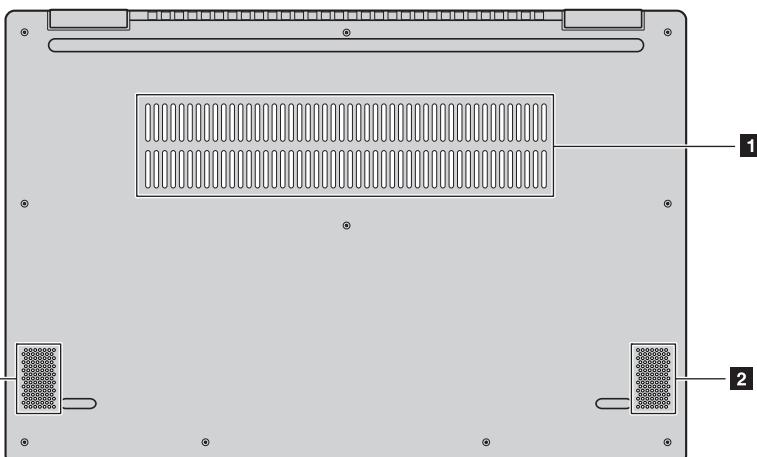
**1 Louvers** Allow air to enter the computer for cooling.
