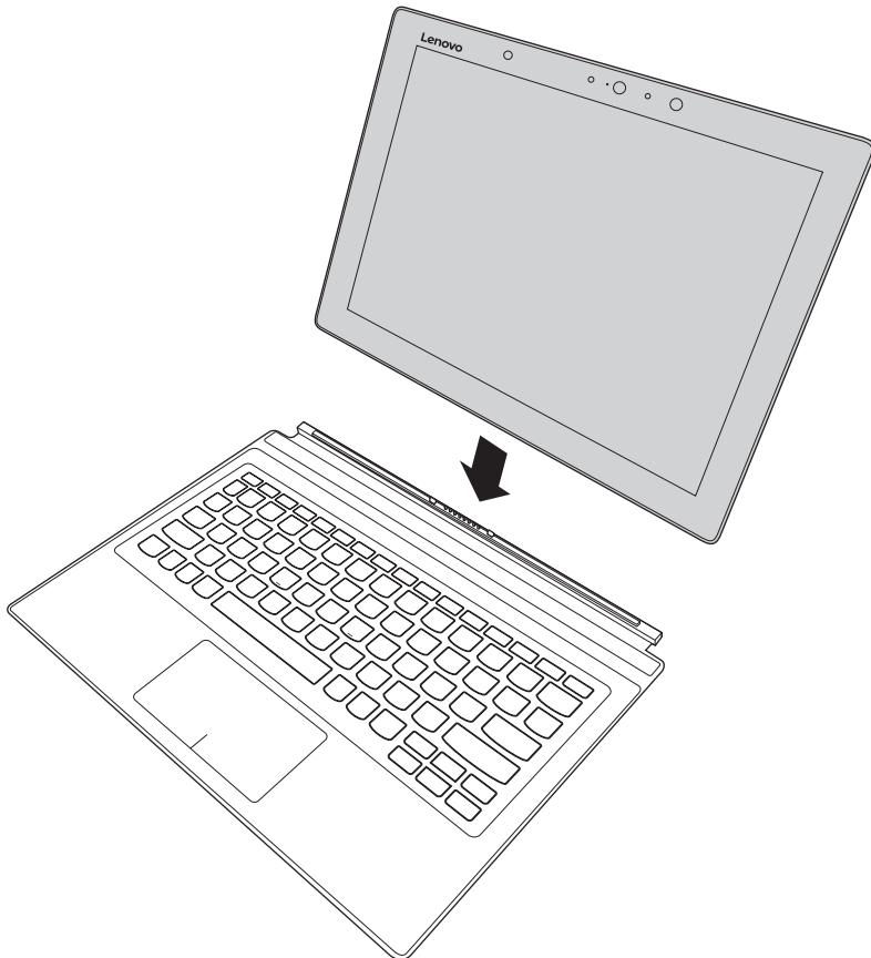
**Note:** Tablet-keyboard folio tongue has strong magnetic force, so as to easily connect with and secure the tablet.
