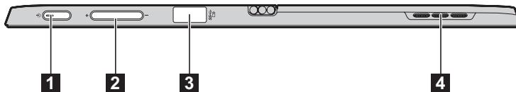
**1 Power button** When the computer is off, press and hold this button to turn on the computer.
