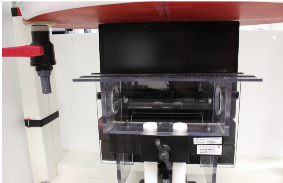
**Top Edge (Laptop slightly open, screen top border totally in contact with the phantom)**
