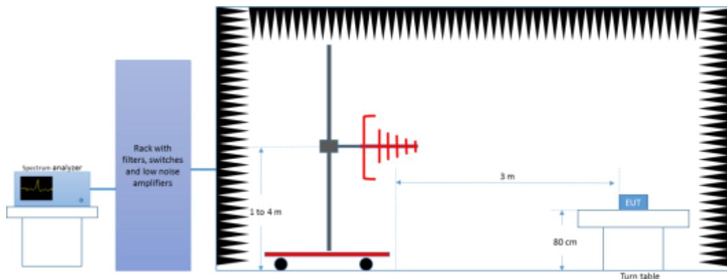
*Radiated Setup 1GHz - 18GHz*
