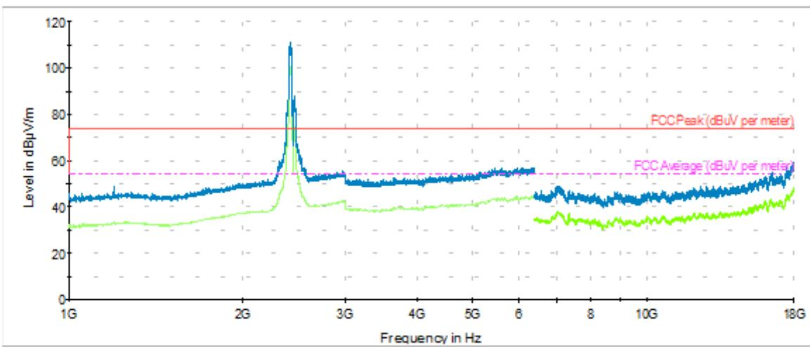
Legend: Peak measurements (Blue line), AVG measurements (Green line), Limit FCC Peak (Red line), Limit FCC Avg (Purple line)
