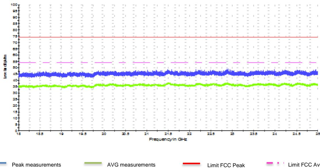
— Peak measurements      — AVG measurements      — Limit FCC Peak      — Limit FCC Avg
