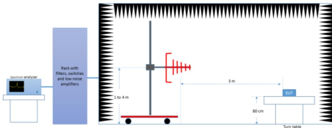
*Radiated Setup 1GHz - 18GHz*
