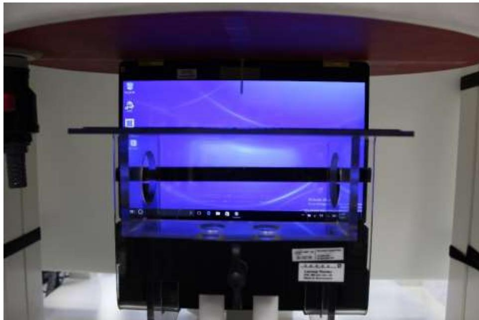
**Bottom Edge (Laptop slightly open, screen bottom border totally in contact with the phantom)**
