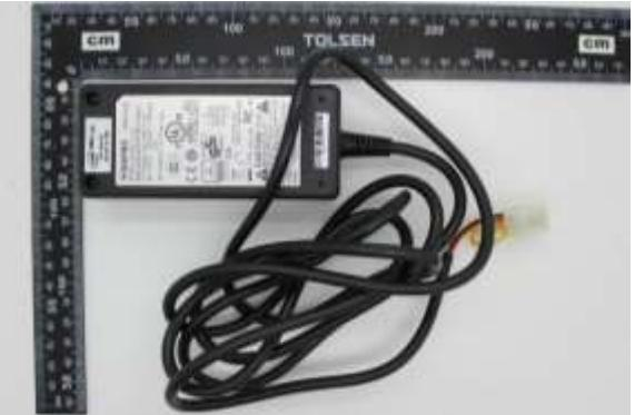
A photograph of a black switching power supply unit (PSU) with a long black power cord. The PSU is positioned next to a metric ruler.                                                          |
