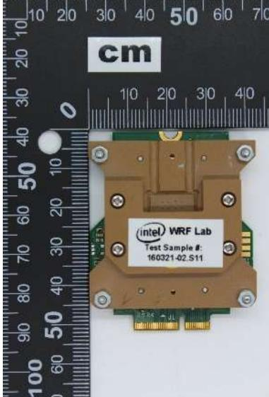
A photograph of a WiFi socket (S11) placed next to a metric ruler. The socket is a green printed circuit board with a gold-plated edge connector. A small white label on the board reads "intel WRF Lab Test Sample #: 160321-02.S11". The ruler shows markings from 0 to 100 cm. |
